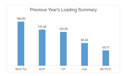
The Non-Coincident Peak Demand is 131.02 MW, which is around 81.89% of the total substation capacity of 160 MVA at a power factor of 0.97. The load factor or the ratio between the Average Load of 82.42 MW and the Non-coincident Peak Demand is 62.91%. A safe estimate of the true minimum load is the fifth percentile of 55.77 MW which is 42.57% of the Non-coincident Peak Demand.
